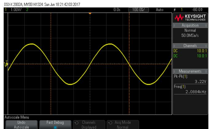
Fig. 10: Oscilloscope output at 2093Hz at 64 Samples
