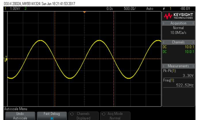
Fig. 9: Oscilloscope output at 523.3Hz at 256 Samples
