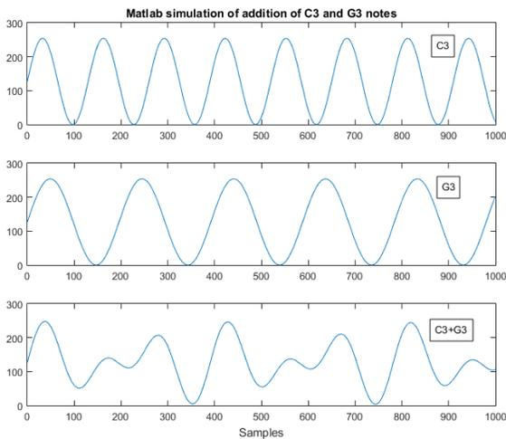
Fig. 13: MatLab Simulation of  $C_3, G_3$ , and  $C_3 + G_3$
