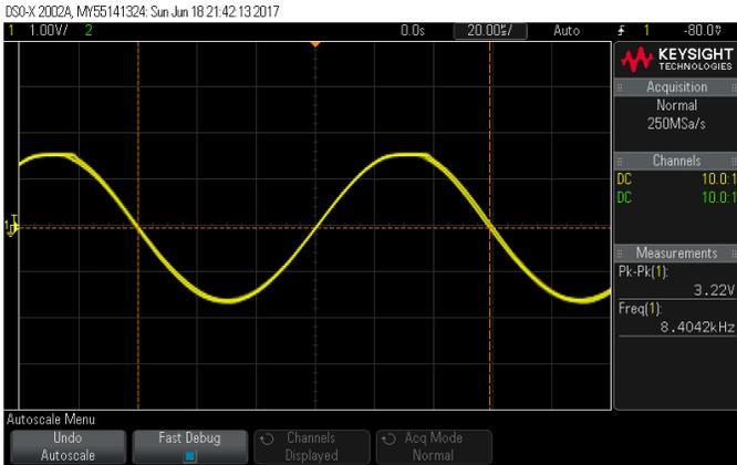
Fig. 11: Oscilloscope output at 8372Hz at 16 Samples
