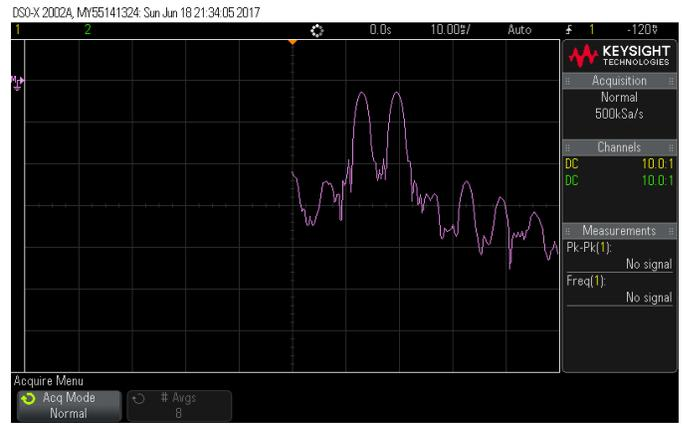
Fig. 14: Fourier Analysis showing the two Peaks:  $P_1$  centered at 130.8Hz.  $P_2$  centered at 196.0Hz.
