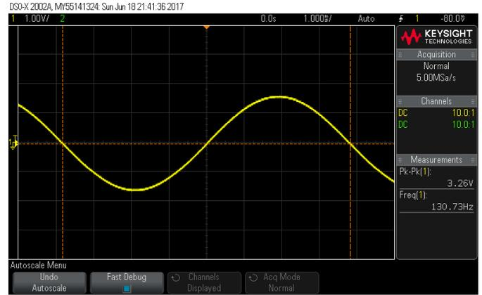
Fig. 8: Oscilloscope output at 130.8Hz at 1024 Samples
