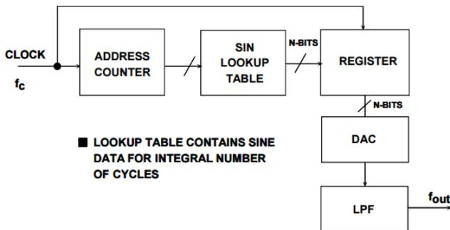
Fig. 1: Simple DDS Block Diagram [4]
