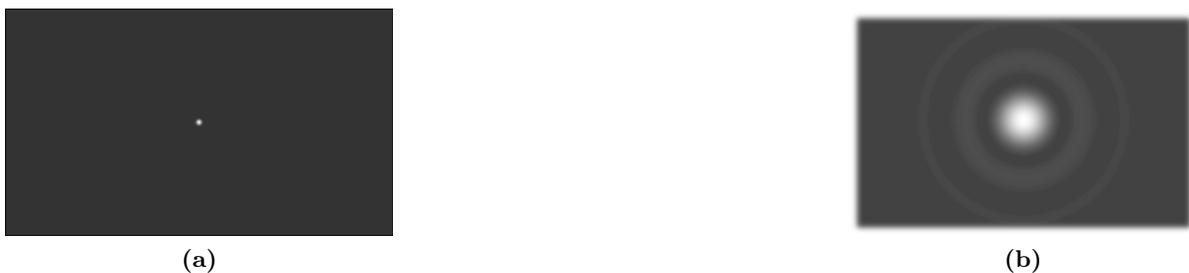
**Figure B.1** – (a) The original point source. (b) The diffracted recording of a point source through a finite sized aperture
