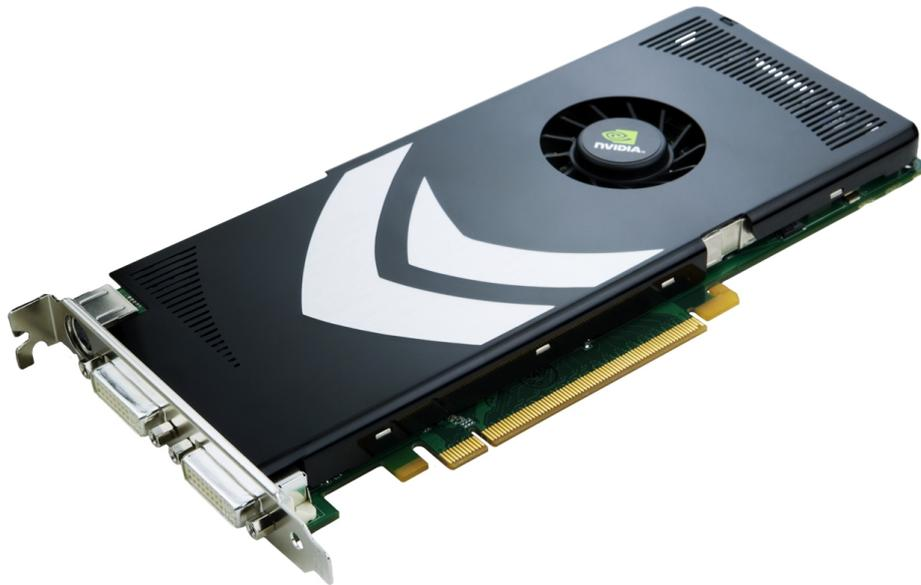
**Figure 3.10** – Nvidia 9800GT Reference Board [56]
