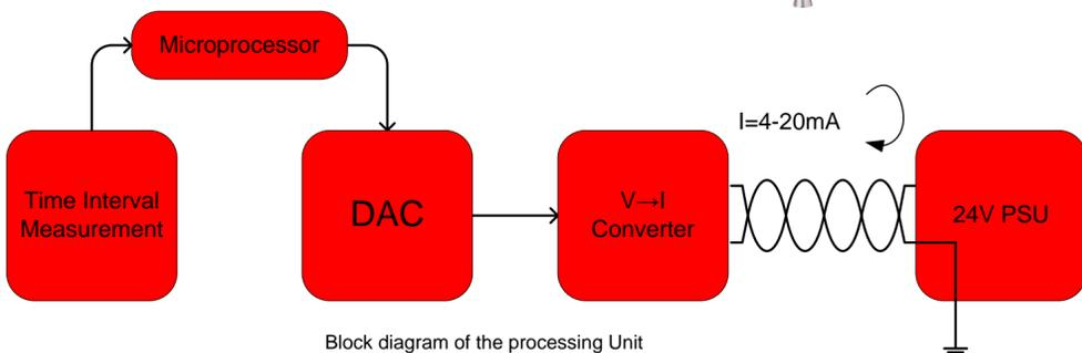
The microprocessor is responsible for controlling the instrument. It is responsible for taking in and co-ordinating time interval measurement. It uses this information to calculate the level which it displays and converts to a digital value. It then passes this value to a digital to analogue converter. The digital to analogue converter then sends a voltage to a voltage to current converter which is responsible for modifying the current on the loop of the supply.
