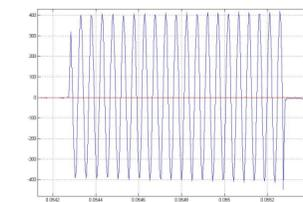
Fed back output showing the USRP capturing the transmitted pulse
