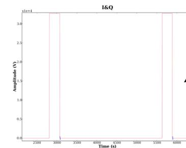
Raw received data showing the PRI triggered marker samples
