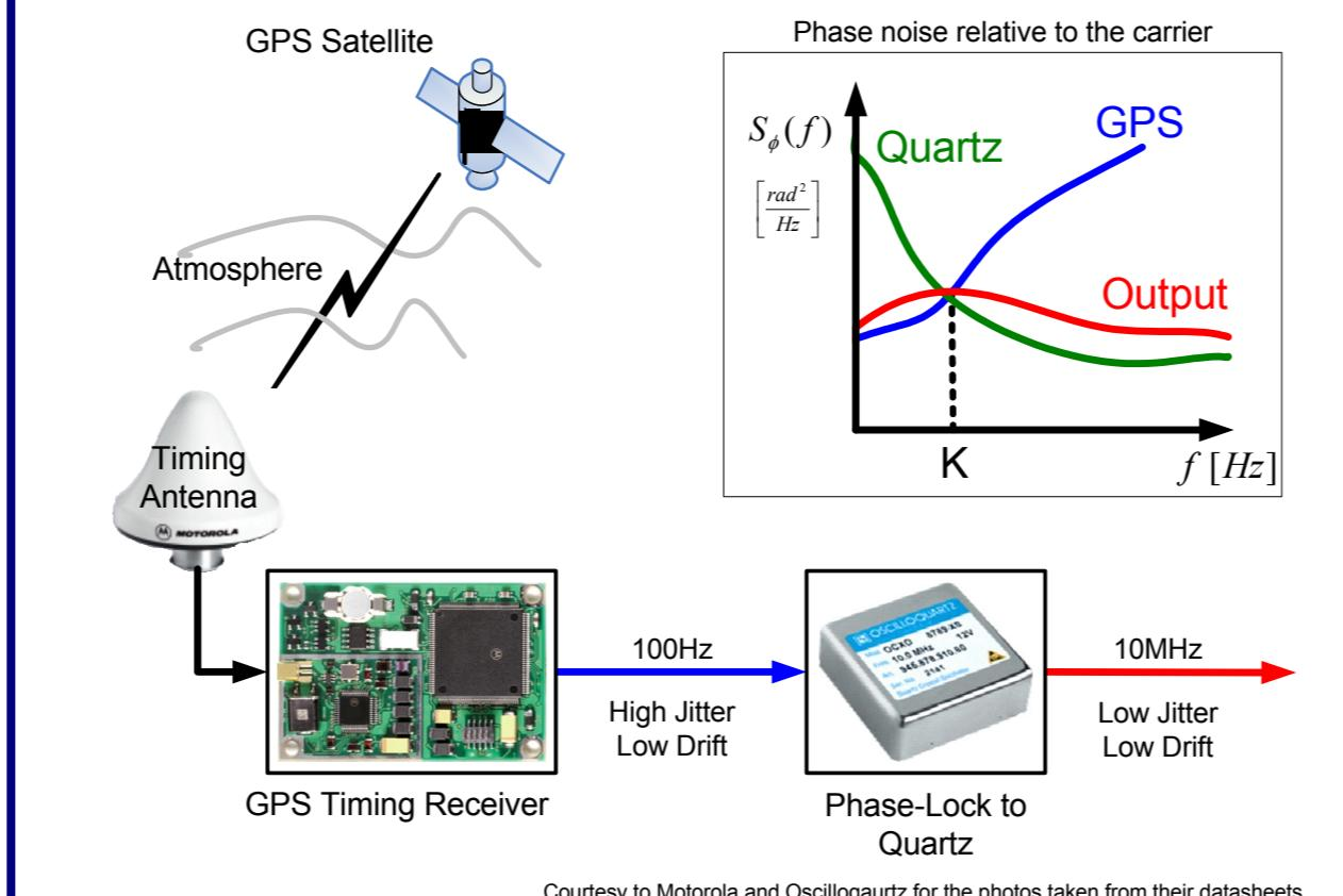
The high frequency jitter that is present in the GPS time mark is filtered by locking it to a low phase noise quartz oscillator. This is done by using the hybrid analogue/digital PLL that is shown above and below.
