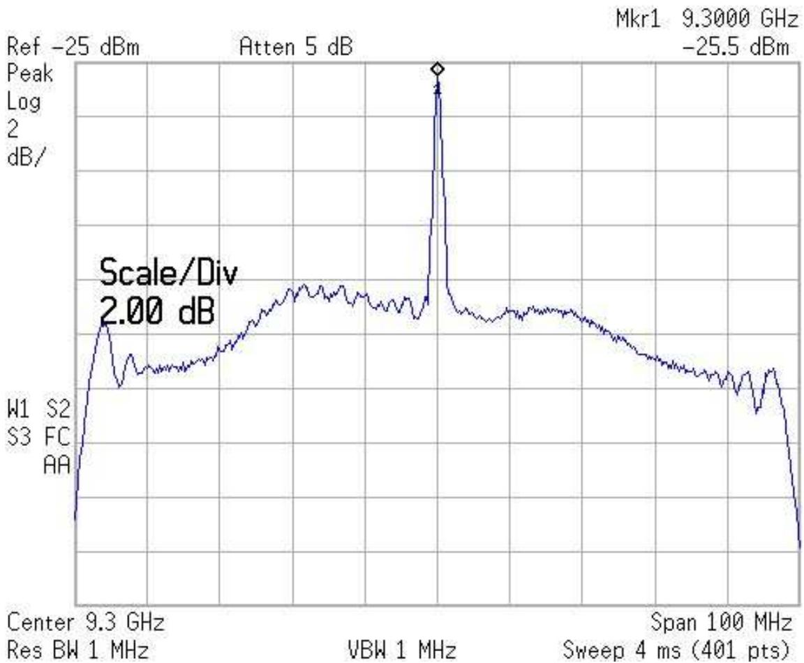
Figure 5.20: Spectrum of 9300 MHz chirp.
