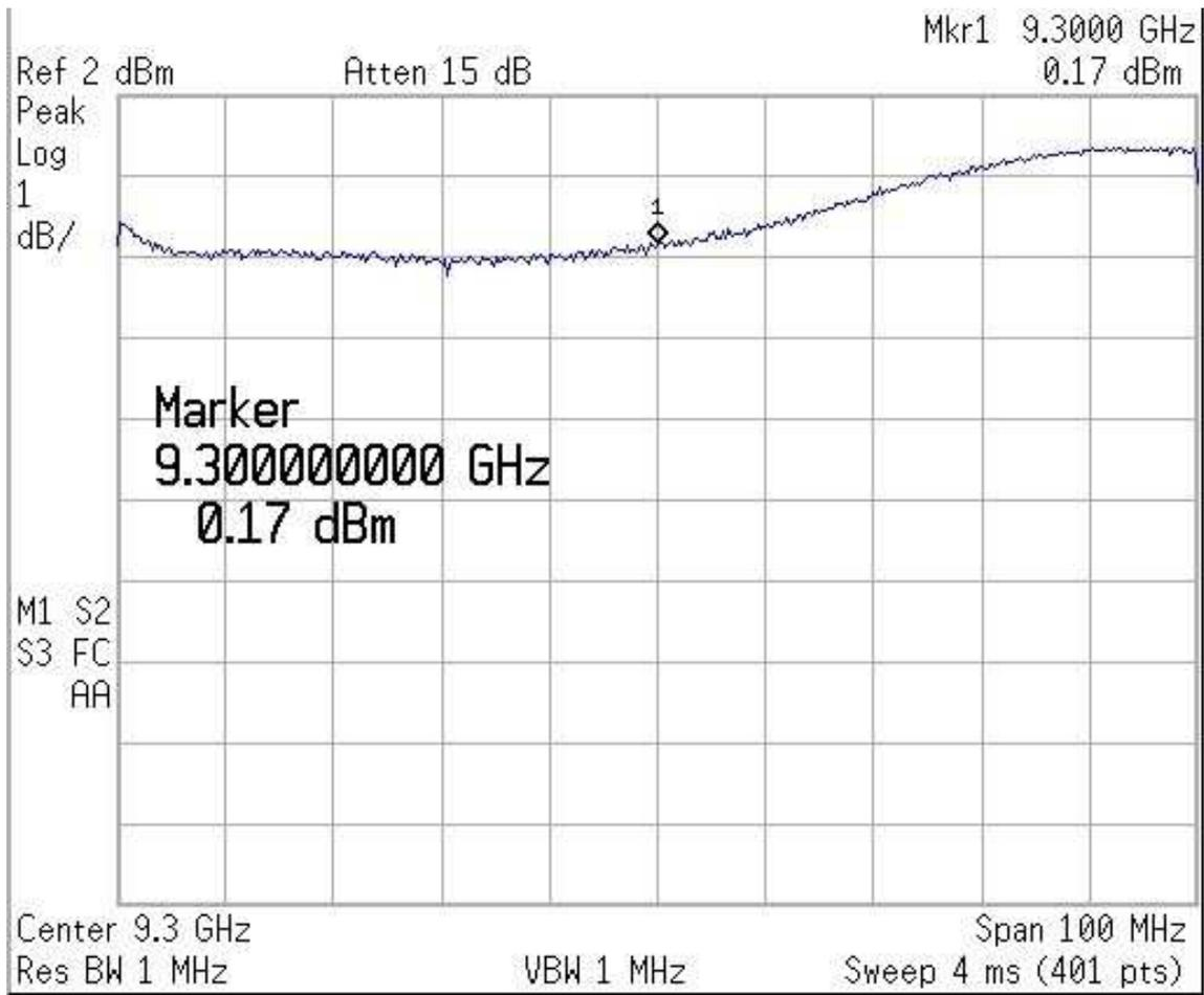
Figure 5.1: Input to transmitter amplifier.
