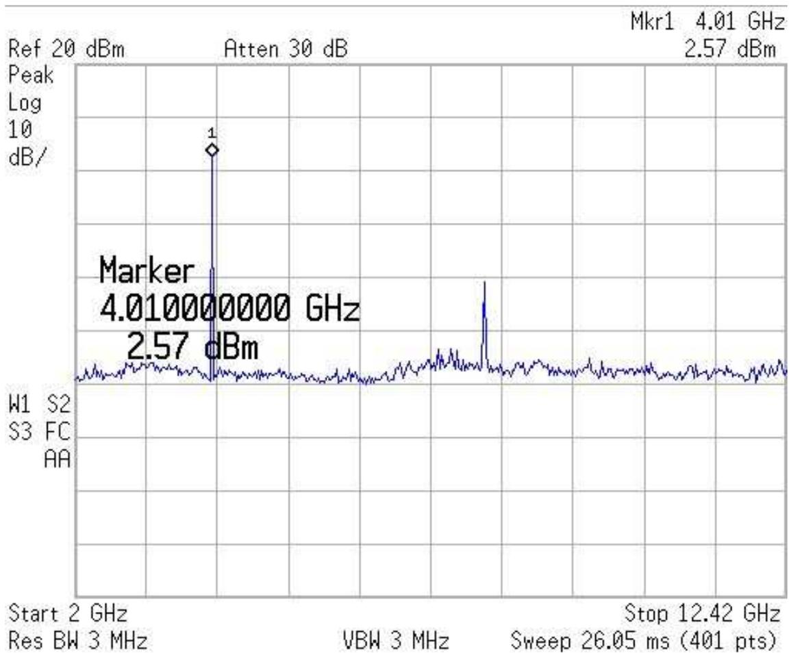
Figure B.6: Plot showing harmonics of the 4000 MHz synthesizer.
