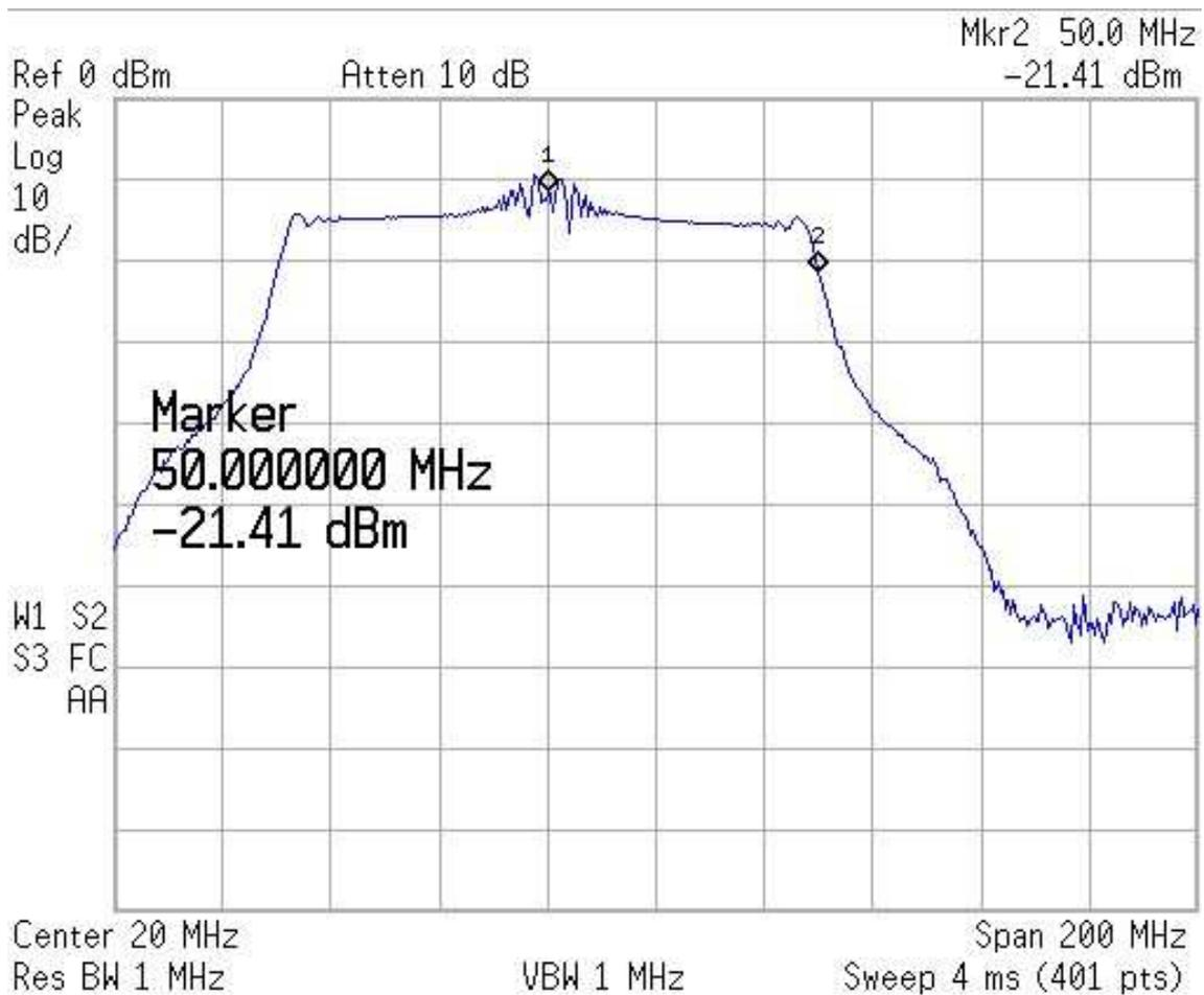
Figure 5.8: Spectrum of baseband in-phase chirp.
