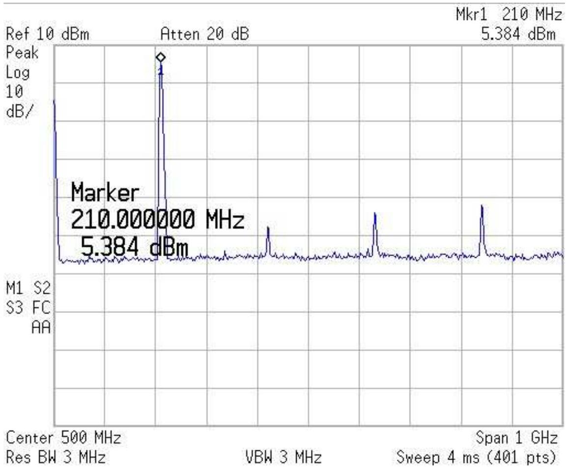
Figure B.10: Plot showing harmonics of the 210 MHz synthesizer.
