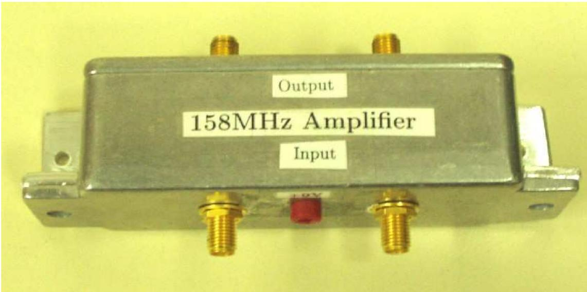
Figure 4.8: Completed module for the 158 MHz amplifiers (AMP11-2 and AMP11-3).
