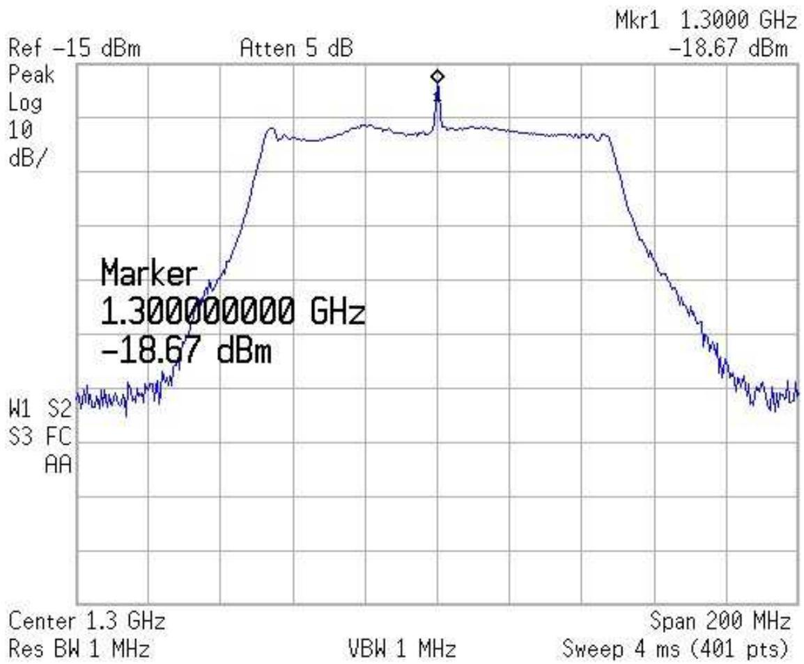
Figure 5.11: Spectrum of 1300 MHz chirp.
