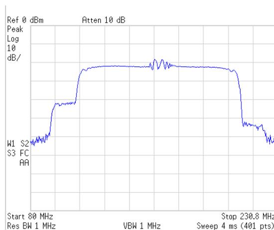
Figure 5.12: Spurious signals in the frequency domain of the 1<sup>st</sup> IF
