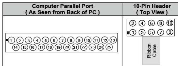
Figure 9: National Semiconductor pin-outs and cable connectors
