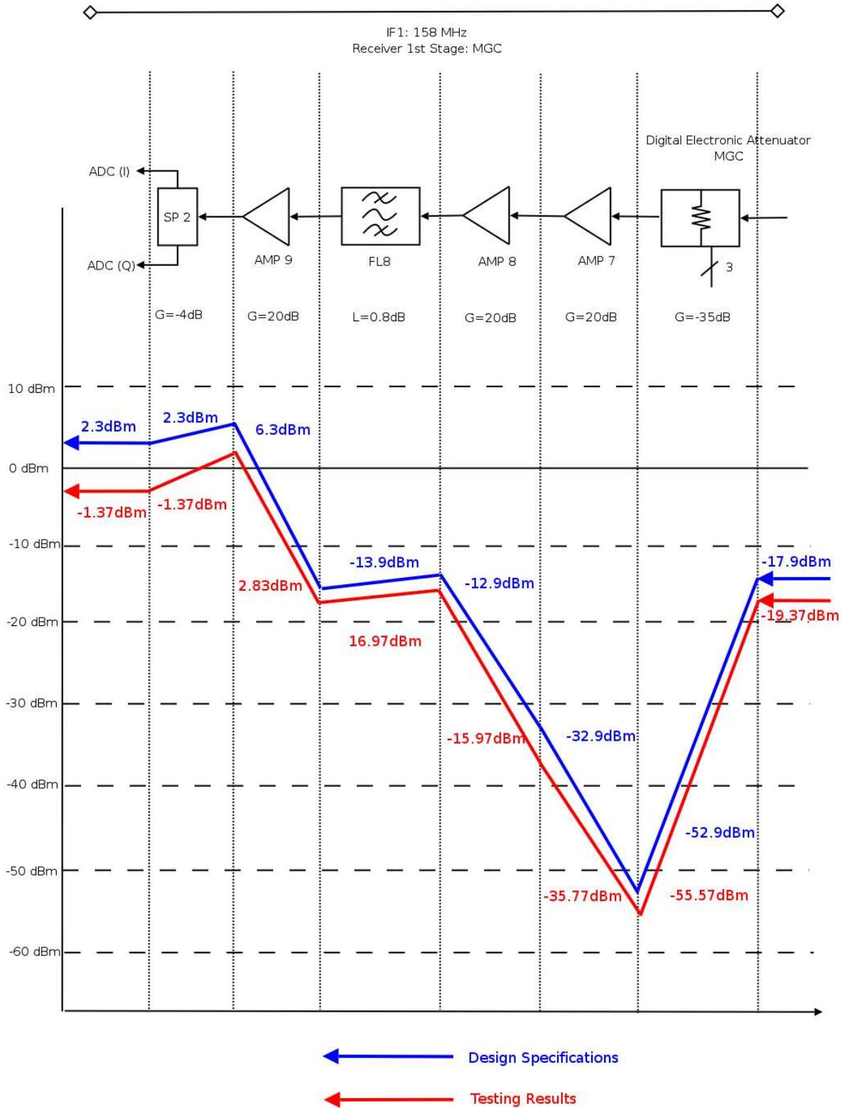
Figure 5.26: Receiver MGC component power levels (MGC max attenuation of -35dB)
