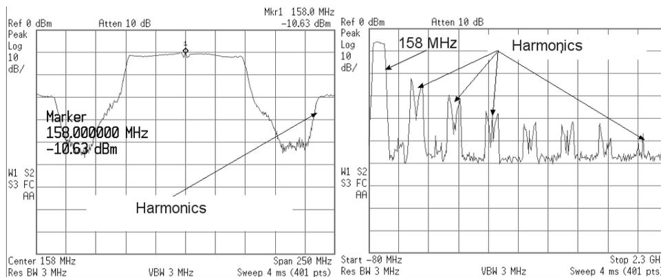
Figure 7.3: IF and LO leakage at SP1
