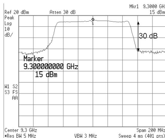
Figure 7.1: RF transmit power with 15 dB gain correction
