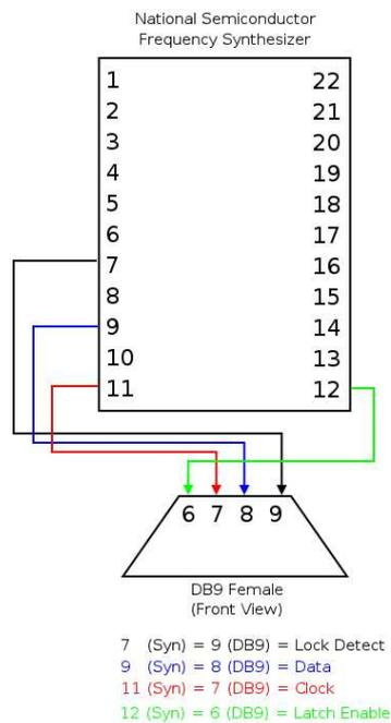
Figure 11: Synthesizer pin-outs
