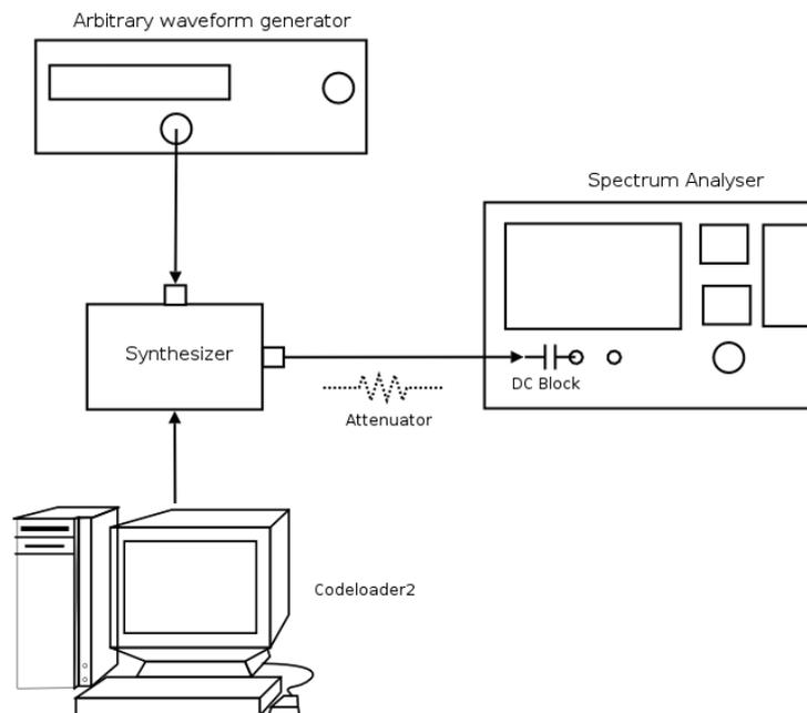
Figure 5.1: FDU testing setup
