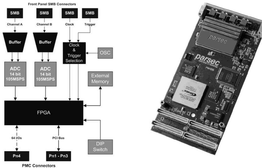
Figure 3.15: PM480 system block diagram, physical PMC card
