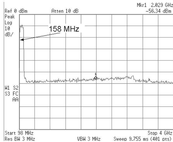
Figure 7.7: Adding additional filter after gain stage
