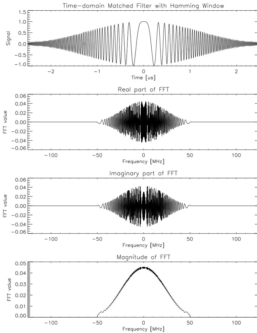
Figure 2.4: Matched filter with a Hamming window
