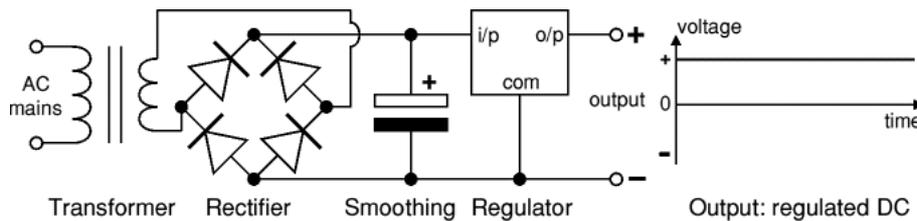
Figure 4.6: Transformer regulatory system
