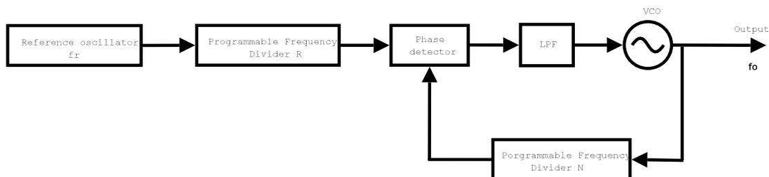
Figure 3.5: Block diagram of frequency synthesis
