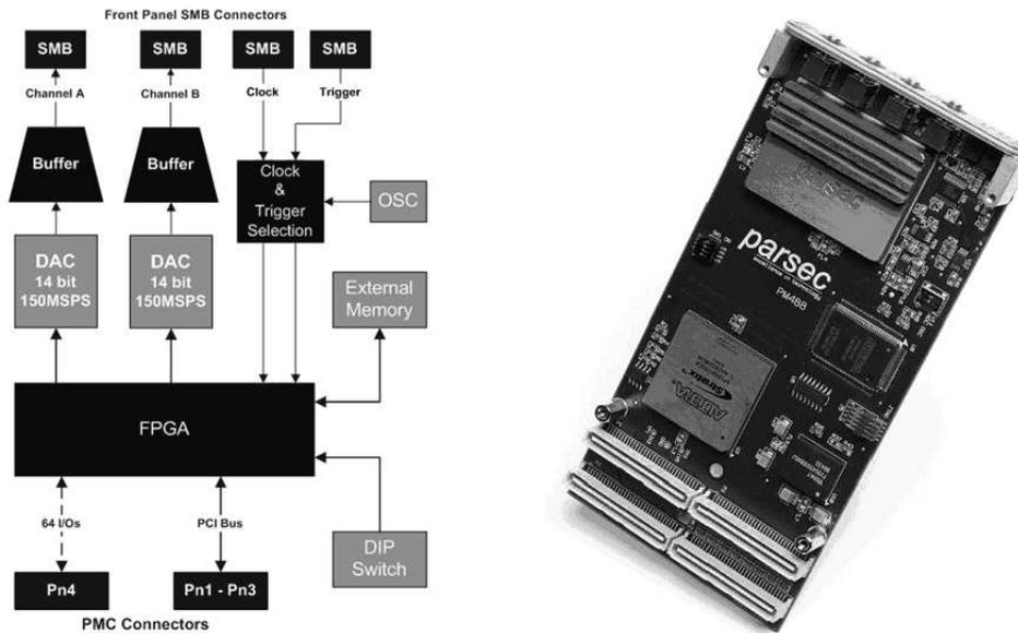
Figure 3.14: PM488 system block diagram, physical PMC card
