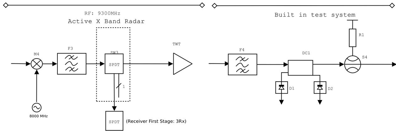
Figure 3.4: Transmitter RF and BIT
