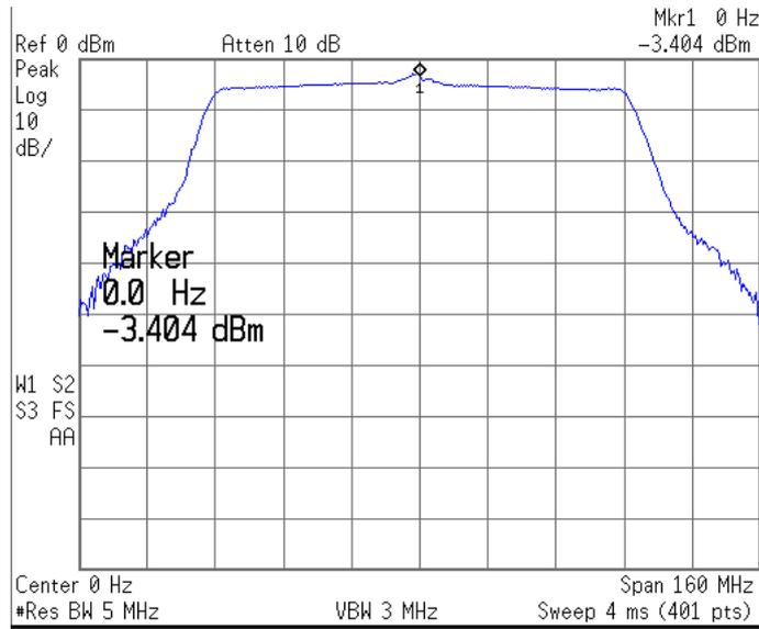
Figure 5.3: Frequency domain band-limiting
