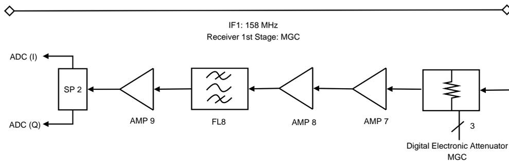
Figure 3.12: Receiver 1<sup>st</sup> IF, Manual Gain Control (MGC)
