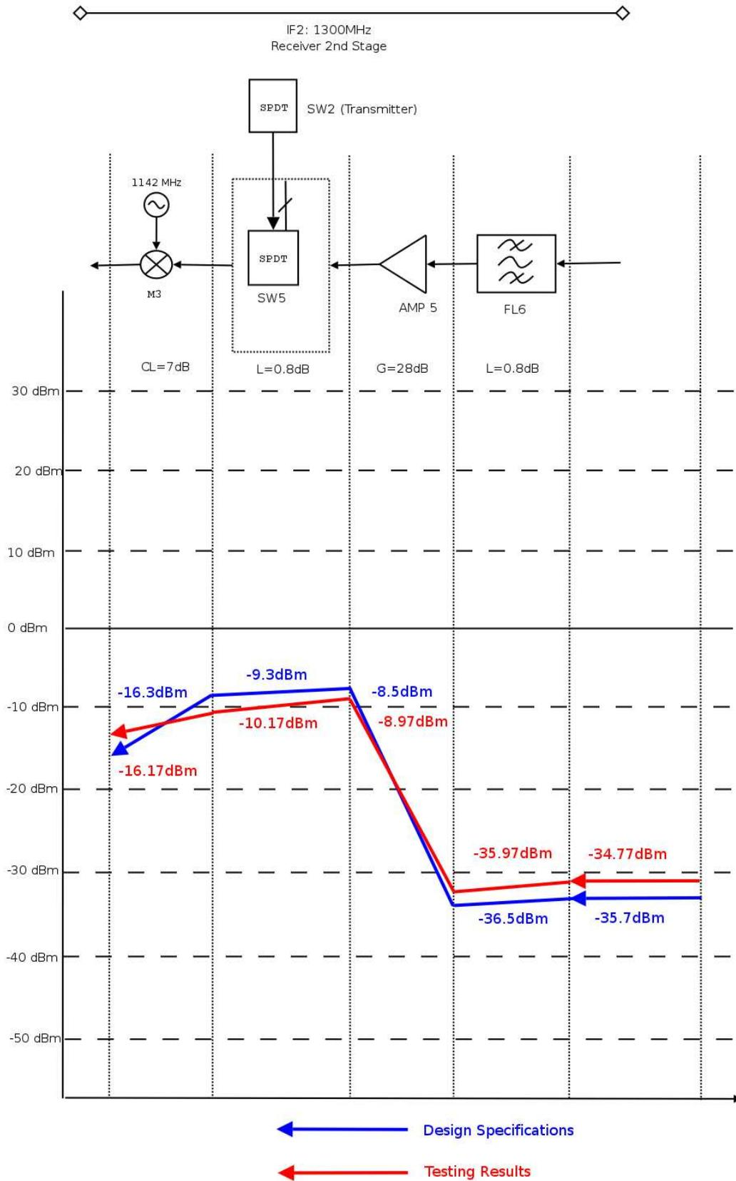
Figure 5.23: Receiver 2<sup>nd</sup> IF component power level
