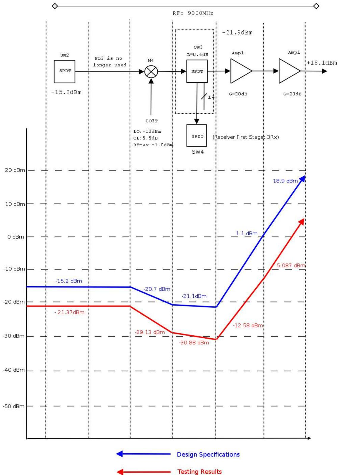
Figure 5.20: Transmitter RF component power levels
