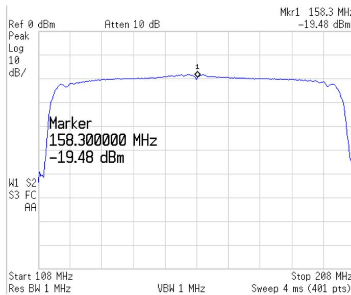
Figure 5.15: 1<sup>st</sup> IF with spurious signals filtered out
