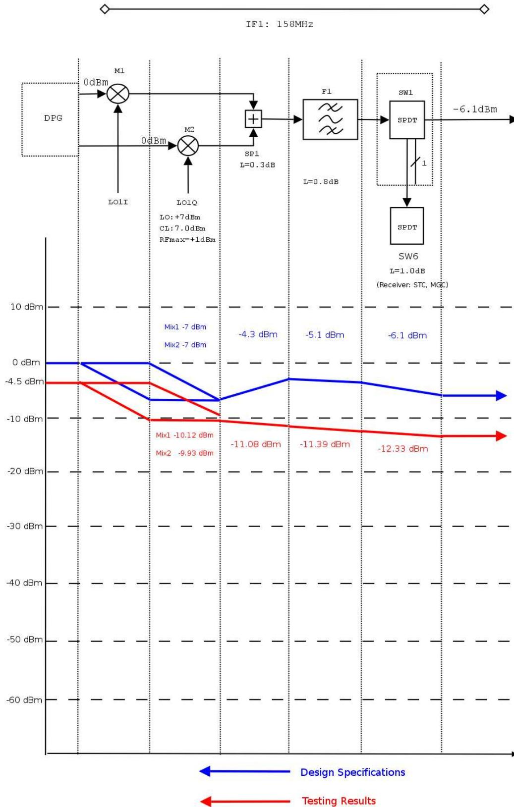
Figure 5.18: Transmitter IF1 component power levels
