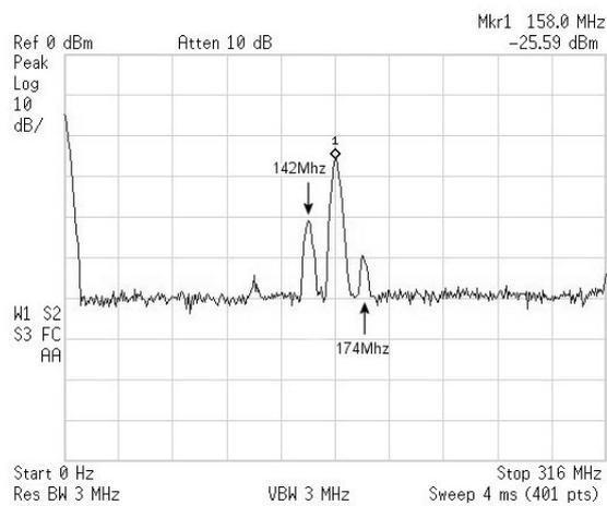
Figure 5.13: Spurious signals at 142 MHz and 174 MHz with IF signal at 158 MHz
