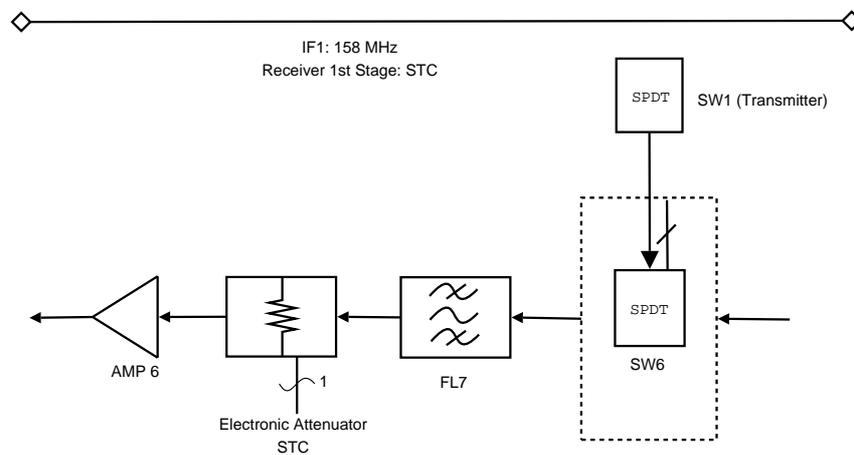
Figure 3.10: Receiver 1<sup>st</sup> IF, Sensitivity Time Control (STC)
