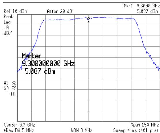
Figure 5.17: RF (9300 MHz) output
