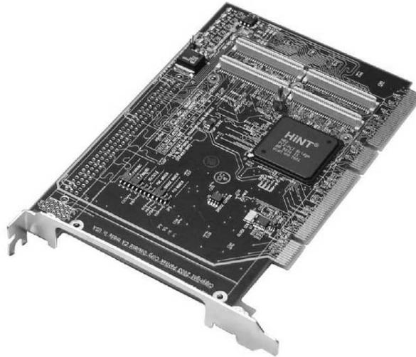
Figure 4.5: Peritek active PMC to PCI adapter card
