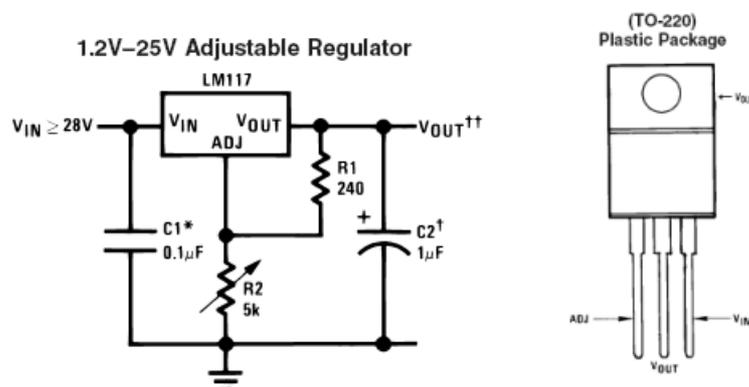
Figure 4.7: LM317/117 variable voltage regulator
