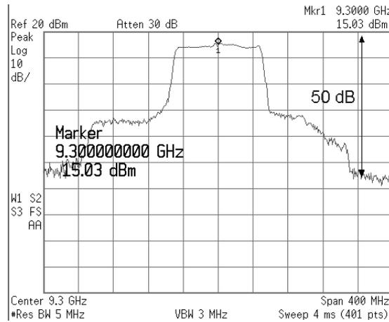
Figure 7.2: RF signal aliased with LO harmonics
