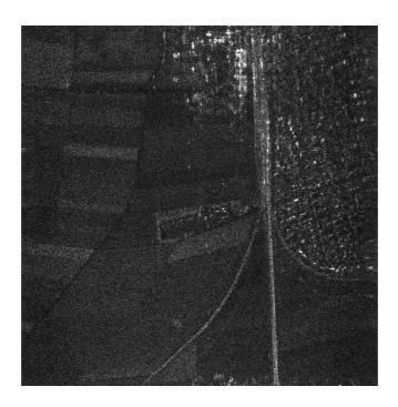
**Figure 2.8:** Single-look E-SAR image obtained using five frequency steps, with  $B_t = 100 \, \text{MHz}$ .
