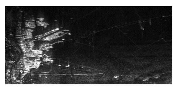
Figure 4.16: VHF-band image after applying the LMS adaptive filter to suppress RF interference.
