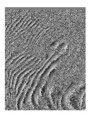
Figure C.15: Interferogram of Hermanus area, with fringes clearly visible.
