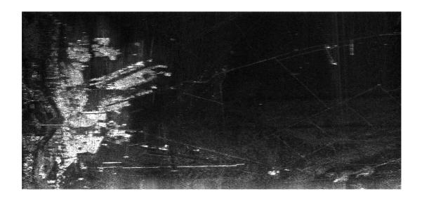
Figure D.2: Cleaned image with weights updated every 100 range lines.
